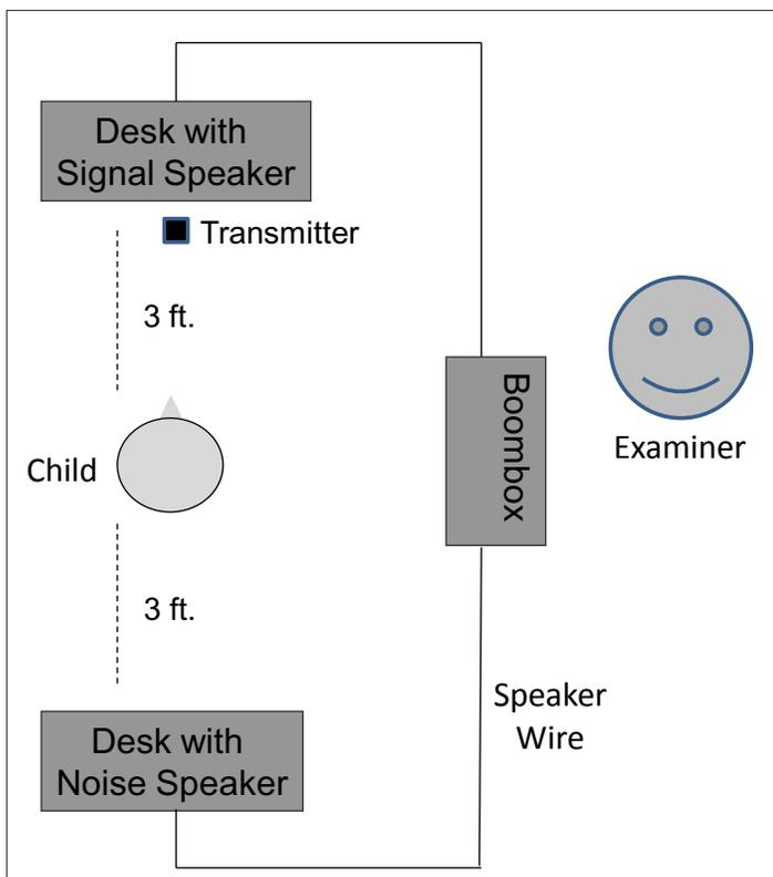
**Figure 1.** Simple equipment arrangement for conducting speech perception testing in noise in a classroom.
