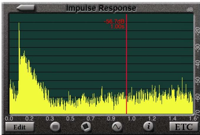
Figure 4. Energy time curve of an unoccupied classroom.
